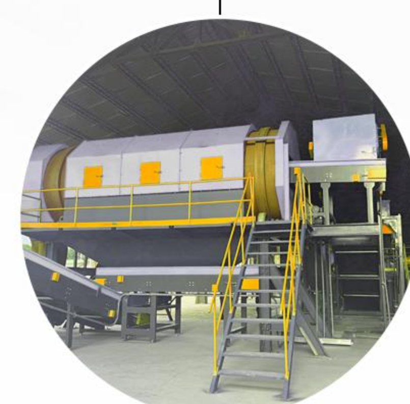
滚筒筛 筛选出物料中的石子等杂质 Rotary Screen Screen out impurities such as stones in the material
